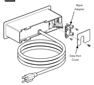
Install Data Port Option (VGA, RJ45, HDMI, BLANK)
