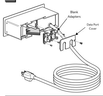
Install Data Port Options (VGA, RJ45, HDMI, BLANK)
