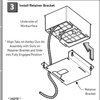
Route Conduit Through Notch in Retainer Bracket
