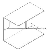
2. Slide end cap over unit as shown. Press firmly to adhere tape.
