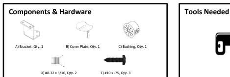
FOR USE WITH: This product fits 2" (50.8mm) - 3.15" (80mm) openings and table thicknesses of 1" (25.4mm) - 1.5" (38.3mm). \*Take care not to pierce finished surfaces with mounting hardware.
