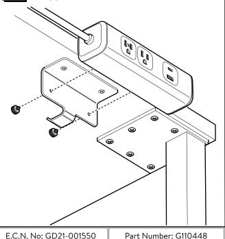
Plug POWER TAP into Powered Outlet and Manage
