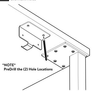
Install POWER TAP BRACKET to Worksurface
