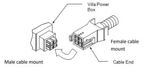
**4-** Slide safety cover (E) onto open male cable mount if desired.
