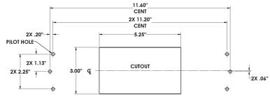
**2-** Mount Villa II (A) beneath the cutout. Secure with screws (B)\* and position as needed. Do not use provided screws on table thicknesses less than 1.00".
