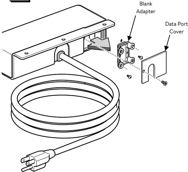
**2 Install Data Port Option - (VGA, RJ45, HDMI, BLANK)**
