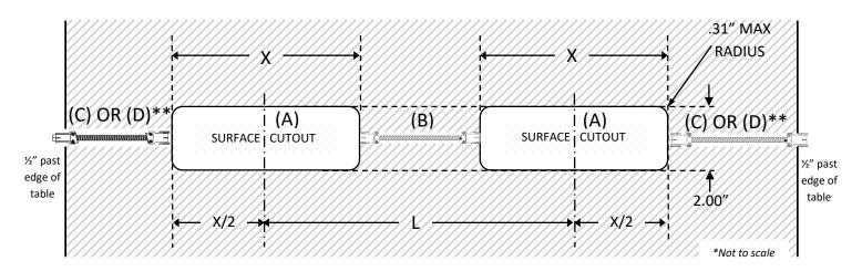
\*\*If (C) Female/Female cable is used on the leftmost connection, it must consistently be used on the leftmost connection while (D) Female/Male cable must be consistently used on the rightmost connection.
