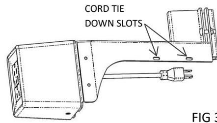
NOTE: A furniture Power Distribution Unit is not for permanent installation as part of the building structure and not for mounting in permanently-installed furnishing such as a fixed countertop.
