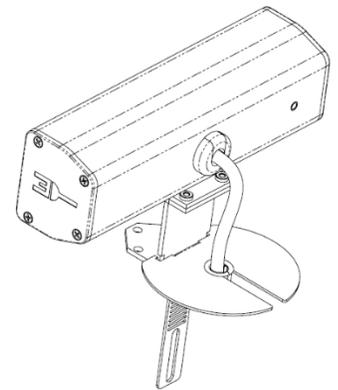
**3-** Insert the cord then bracket (A) through table opening. Position the Seclusion to the front of the table opening and secure bracket to underside of table using 2 screws (E)\*.
