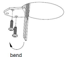
**4-** Ensure the cover plate (B) is fully seated on the table, hold in place while bending cover tab flat against the bracket as shown. Insert the remaining screw (E)\* to secure.
