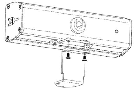
**2-** Slide the cover plate (B) onto the bracket (A) and attach the cord to the split bushing (C). Feed the cord through the cover plate slot and seat the bushing.
