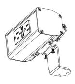
**2-** Insert the cable through table opening. Position the Seclusion and secure bracket to the table using 2 screws.
