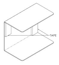
2. Slide end cap over unit as shown. Press firmly to adhere tape.
